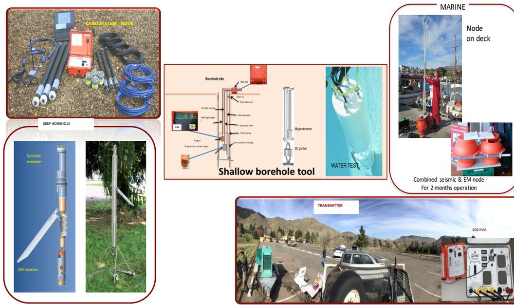
FIGURE 1: System hardware examples for the multi-physics array electromagnetic system.
