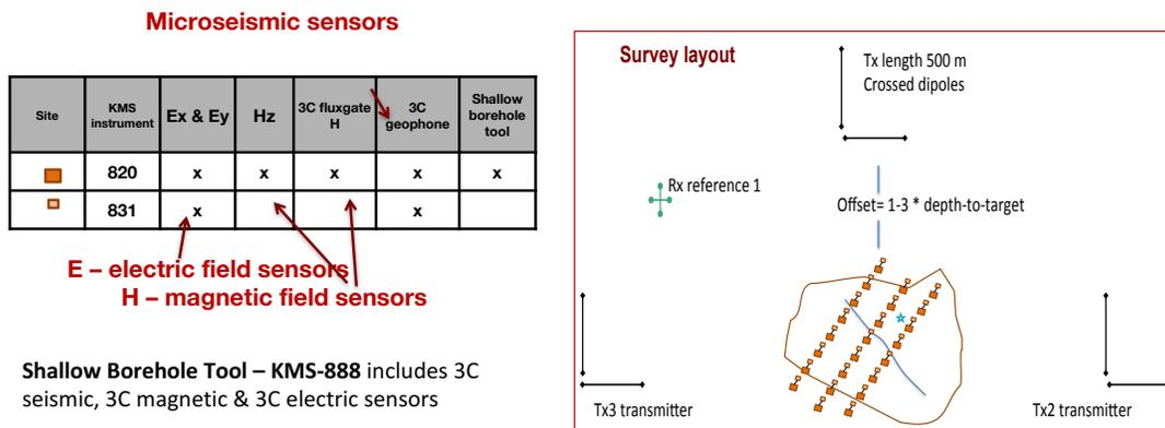
FIGURE 2. Generic survey layout for monitoring applications for a flood front using multi-physics geophysical sensors.
